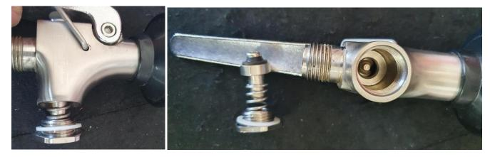
STEP THREE (3) – Do reverse process to assemble. Push Hex Male against the spring and turn to screw into body. Tighten up tightly.
