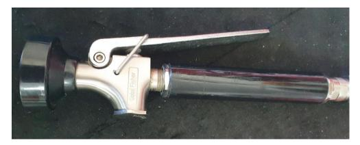
STEP ONE (1) - Unscrew the Hex Male underside of squeeze lever. <u>CAUTION</u> - this is spring loaded.
